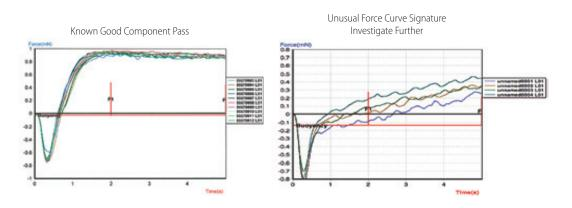
It is the superior force measurement sensitivity of the MUST 3 that produces a very distinctive force curve signature. Comparing the signature obtained from testing a known good component and comparing any signature change provides a clear indication of the need for further investigation.
