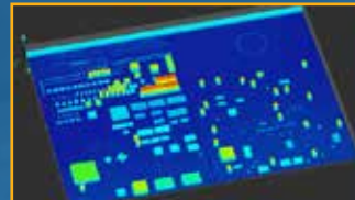
Whole Board 3D Data Flatness measurement
