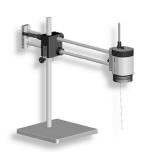
**OP-006 199 is a heavy duty and stable stand with precision ball-bearing boom movement**, specially developed for using with W10x High Definition and PAL range of Optilia inspection cameras. Working range and Object distance of the camera can be precisely adjusted and locked by a grip knob. An optional 4-directional tilt unit can be assembled on front of the boom in order to change direction angle of the camera for side inspection of objects.
