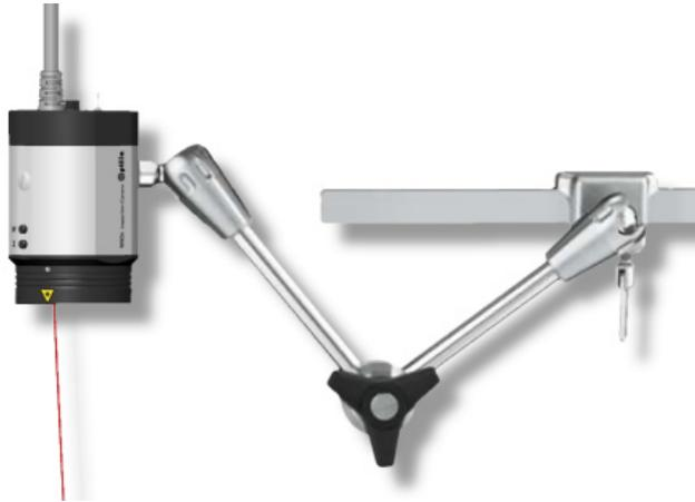
Articulated arms can be positioned easily and precisely in any position. All three joints are fixed steady with the central tightening knob. The quick lock and the step-less tensioning system assure ease of use and allow efficient working.
