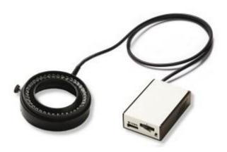
Ring-light containing 40 white LEDs for bright and homogenous illumination of objects. Designed for assembly on Optilia W10x-HD, W20x-HD and M20x-HD cameras. The compact control unit features an ON-OFF switch, brightness control and two outputs for connection to LED illumination units. With Segment control unit, user can toggle 4 groups of LEDs clockwise or anticlockwise.
