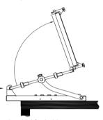
Foam rubber-lined lid for holding components in place. May be raised by applying pressure to front buttons.
